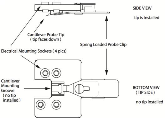
Note | The electrical mounting sockets are not equally spaced. Only one particular orientation is allowed for holder mounting. Do not force the holder to be mount in a wrong orientation or it will be broken. The holder is not cheap (\$630USD)
