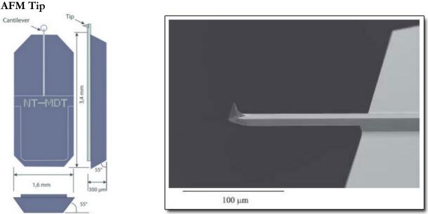
The AFM tip/cantilever locates at the end of the alignment mark on a probe chip. Always face the alignment mark up or the tip/cantilever will be destroyed.
