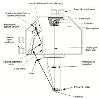
There are four knobs on the scanner -2 for laser aim adjustments (x and y) and 2 for detector mirror position adjustments (x and y). The tip holder is mounted on the bottom of the scanner.
